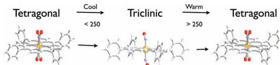
Figure 4. Diagram illustrating the changes in the solid-state structure of [\text{Fe}(\text{TPP})(\text{NO})] as the crystalline sample is warmed and cooled. Reproduced from ref 22.
